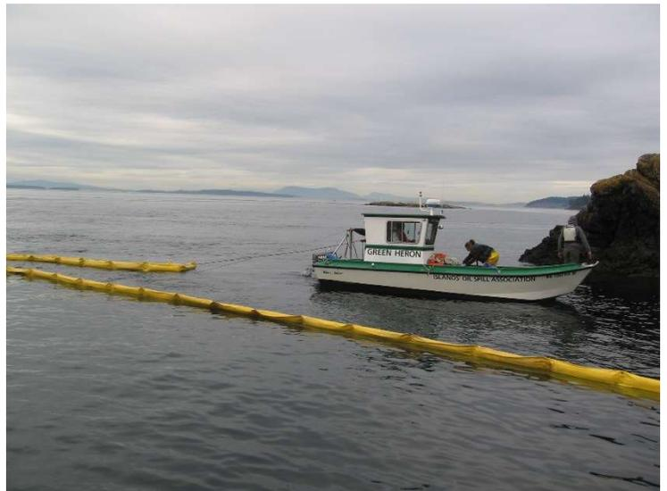
*IOSA response boat Green Heron tows oil containment boom to an attachment point during an oil containment drill in Small Pox Bay on the west side of San Juan Island.*
